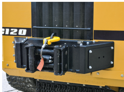
Hydraulic rear winch with 12,000-pound capacity.
